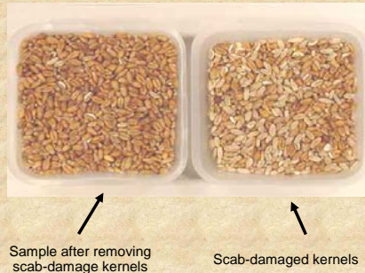
Figure 2. Samples after separating healthy kernels from scab-damaged kernels using a single-kernel near-infrared sorting system
